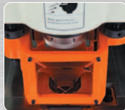
*Laser alignment system for more accurate positioning of marked parts.
